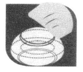
(4)Replace TOP-COVER Make sure TOP-COVER is securely seated on the water container.
